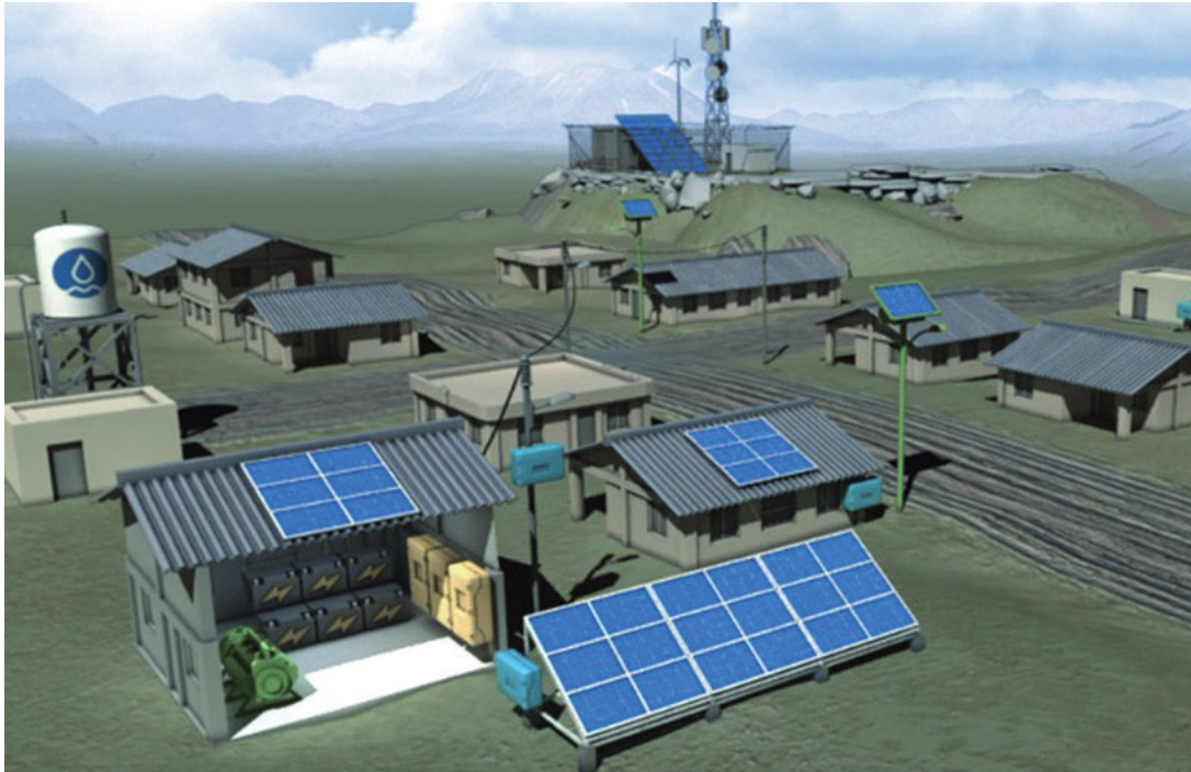
Figure 3.2.1.3.1: Example of a mini-grid with decentralised PV, wind turbines, batteries, a diesel generator and a distribution grid/network. | Source: http://www.ennera.com/en/detail-solution/minigrids .
